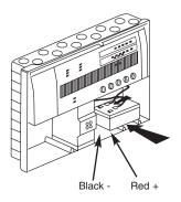
The 8 zone panel requires two batteries (supplied): 2x12v 3.2Ah
