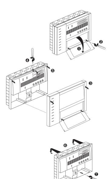
Mount the panel, using pre drilled screw positions, to the wall. This will prevent any possible brick dust contamination of the panel internal circuitry.
