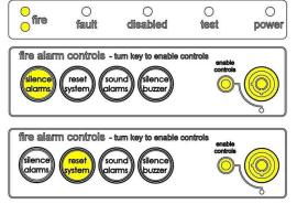
The red 'FIRE' LEDs will illuminate, the fire alarms and the internal buzzer will operate as programmed. Take appropriate action as defined by the emergency plan for the premises.
