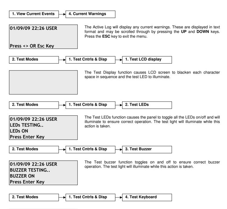
01/09/09 22:26 USER KEYBOARD TESTING.. ENTER key PRESSED. Press Enter Key The Test keyboard function enables the user to select each button to ensure the correct function is shown on the screen. Press the **ESC** key **TWICE** to exit the menu.
