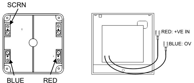
Care should be taken when terminating devices to ensure all cables are correctly sleeved and connections are secure. Improper connections will prevent a system from responding properly in the event of a fire. Please remember that all high voltage testing must be carried out before the installation of the Flashpoint front unit as this may cause damage. It is important to maintain the screen continuity in order to protect against data corruption from interference.
