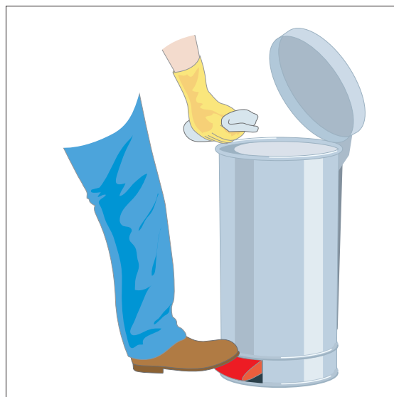
Figure 15: A fire-resisting pedal bin for rags
